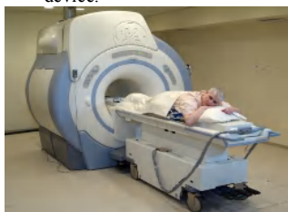
Fig.2 Patient Table -Docks to MR scanner -Consists of electronics and transducer in water bath
